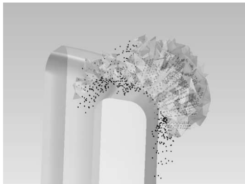
Figure 1: Sketch depicting emission of hot electrons from the tip of a 3D plasmonic nanoelectrode
