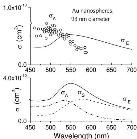
Figure 1: (upper panel) Photoacoustic excitation profile of 93 nm diameter gold nanospheres in aqueous dispersion. (lower panel) Simulated absorption, scattering and extinction cross sections.
