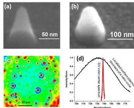
Figure. (a) Platinum based nanocone fabricated by EBID. (b) Gold plasmonic nanocone. (c) SiV color centers in diamond. (d) Spectral matching of plasmon resonance of the nanocone with the SiV color center.
