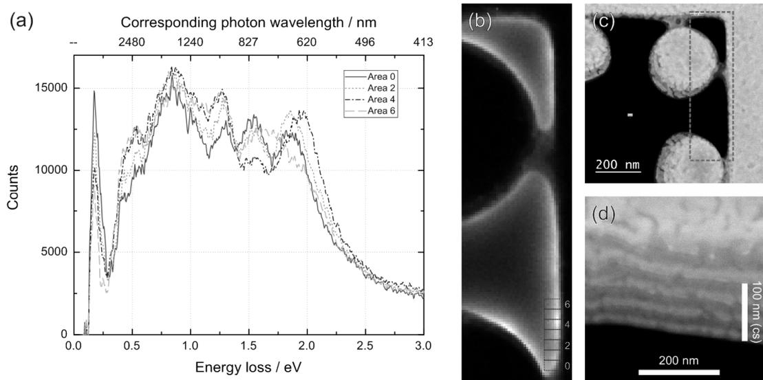
Figure 1: (a) EELS spectra from a HMM Au-Al<sub>2</sub>O<sub>3</sub> multilayer structure at areas marked in the (b) STEM EELS map of energy loss at 1.75-1.85 eV. (c) STEM HAADF image with the EELS image area marked. (d) Scanning electron micrograph of the multilayer edge at a 52° angle.
