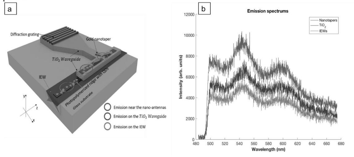
Figure 1: a) The photopolymerized ridge onto the main arm,(orange spheres on the brown layer). The circles represent the areas where it has been used the confocal microscope to collect the emission of QDs into the spectrometer. b)The graph shows the emission in three different cases: close to nanoantennas (blue line), on the TiO<sub>2</sub> ridge (green line), on the IEW (red line).
