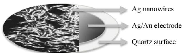
Figure 1: Sensing platform composed of AgNWs (BAM image) transferred on a QCM sensor.
