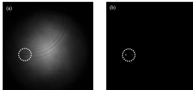
Figure 2 – (a) White light image of the resonating structure. (b) Localized emission from the resonating structure. Light coupling by means of lensed fiber in side-coupling configuration.
