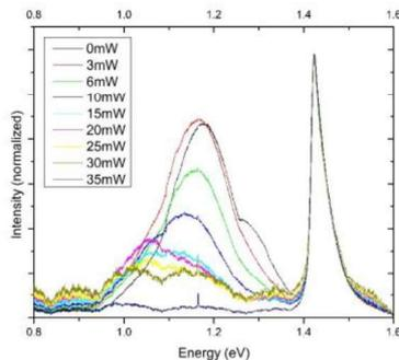
Fig.1. Laser annealing with different powers ranging from  $P=3\text{mW}$  to  $P=35\text{mW}$  for a time period of  $t=7$  seconds.
