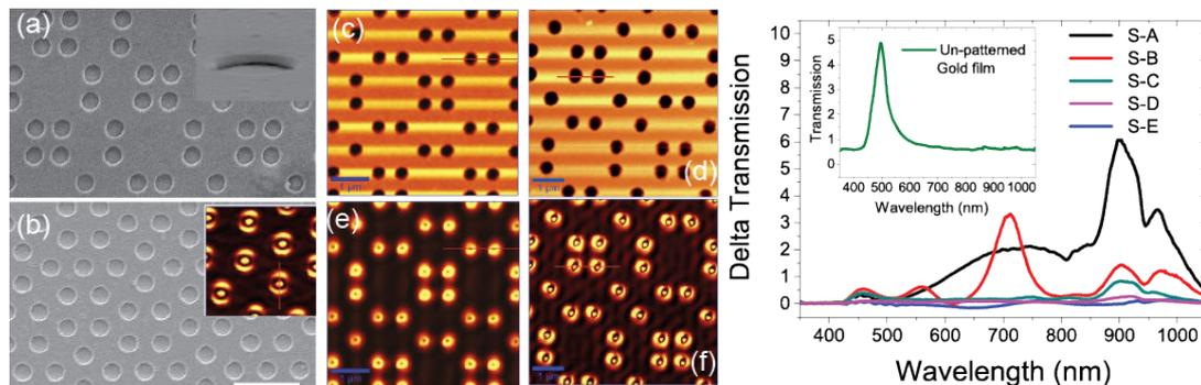
Figure 1: (a)-(b) SEM images of the quasi-periodic nanocavities. (c)-(d) AFM topographic scans of the Thue-Morse nanostructure under different polarization/wavelength excitation. (e)-(f) SNOM images of the Thue-Morse nanostructure under different polarization/wavelength excitation. (g) Enhanced Transmission measurements of the different samples.
