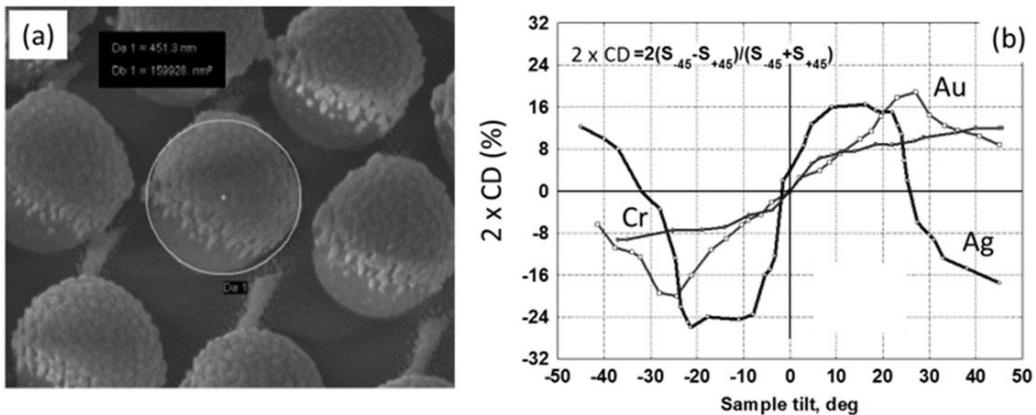
Figure 1: (a) SEM image of the realized metasurface. (b) circular dichroism as a function of incidence angle for different metals (Cr, Ag, Au).
