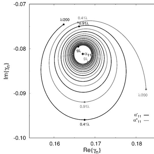
(b) Loci spanned in the complex plane by the dipolar eigenvalues of a dimer of spheres with radius  $\lambda$ , by varying the edge-to-edge distance from  $\lambda/200$  to  $9\lambda$ .
