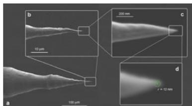
Figure 2: SEM images of a double tapered tip with subsequent zooms ((b), (c) and (d)) on the apical part showing a radius of curvature  $r \sim 12$  nm.
