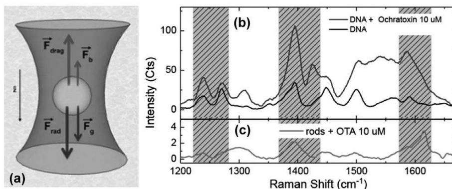
Figure 1: (a) Schematics illustrating all the forces acting on BIO-NRC, approximated here as a sphere. (b) SERS spectra of nanorods functionalized with DNA before (black) and after capture of OTA (gray). (c) Control experiment using non-functionalized rods yield a negligible signal.
