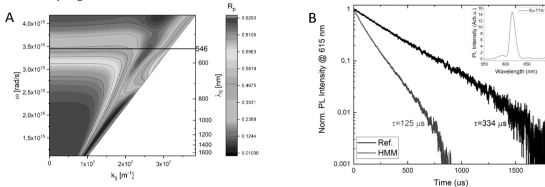
Figure 1: (A) Reflectance simulated spectrum for p-polarized light impinging on a 180 nm thick multilayer composed of four alternating alumina ( $t=30$  nm) and gold ( $t=15$  nm) layers. (B) PL decay curve of EuTTA doped PMMA layer deposited on SiO<sub>2</sub> substrate (Ref.) and on the HMM multilayer.
