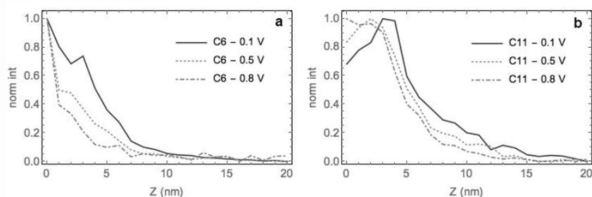
Figure 1: TERS tip-approach curves at different bias voltage for (a) C6 and (b) C11.
