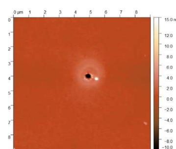
Fig.2. For  $P=35\text{mW}$  and  $t=7\text{seconds}$ , Arsenic (As) desorption happens, and a hole is created (observed by AFM).
