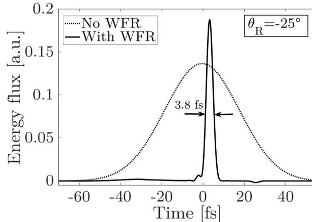
Figure 2: Energy flux of a SPP generated by a WFR pulse compared to one generated without WFR.
