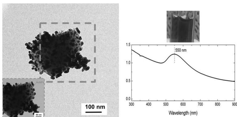
Figure 1: TEM images and UV-VIS absorption spectrum of AuNPs/PEG-DNPs.
