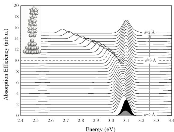
Figure 1: TD-DFTB absorption spectra for a COOH-B-TS molecule put at several distances from an Ag<sub>20</sub> cluster and oriented perpendicularly to the tetrahedron basis.
