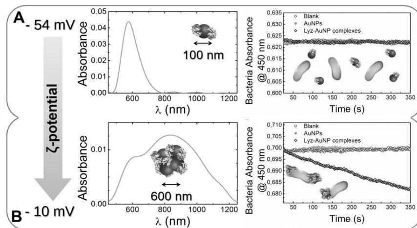
Figure 1: Scheme of the modulation of the properties of Lyz decorated AuNPs complexes at increasing the surface  $\zeta$ -potential; representative absorption spectra and activity assays of single (A) and aggregated (B) AuNPs are shown.
