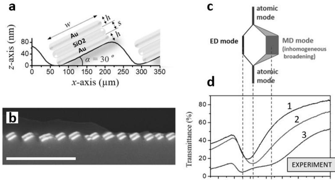
Figure 1: (a) Sketch of Au-silica-Au dimers confined on a faceted ripple pattern;  $w = 100$  nm,  $h = 30$  nm,  $s = 42$  nm. (b) SEM image of Au-silica-Au dimers in cross-section view, scale bar correspond to  $1 \mu\text{m}$ . (d) Cartoon of the hybridization mechanism taking place in the dimer configuration. (e) Optical spectra for transversal polarization (TM) of Au NWs (curve 1), Au-silica NWs (curve 2), Au-silica-Au dimers (curve 3) at normal incidence.
