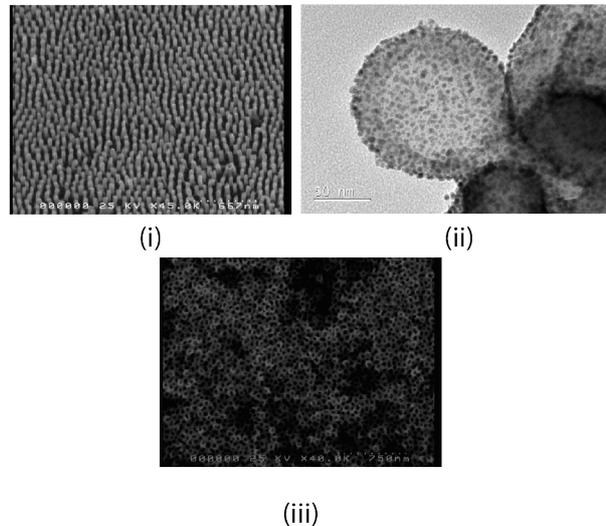
Figure 1: The various geometries analysed: (i) plasmonic nanorods; (ii) silicon nanoparticle with gold coating; (iii) plasmonic nanotubes.
