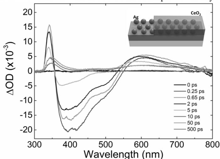
Figure 1: Transient absorption of Ag nanoparticles embedded in CeO<sub>2</sub>.
