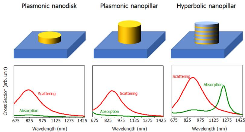
Figure 1: Scattering and absorption cross section of (i) a HMM nanopillar made of 5 bilayers of metal and dielectric on a glass substrate (left-panel), (ii) a classical plasmonic antenna on a glass substrate with the same shape and amount of gold (central-panel) and (iii) the same shape and size (right-panel).
