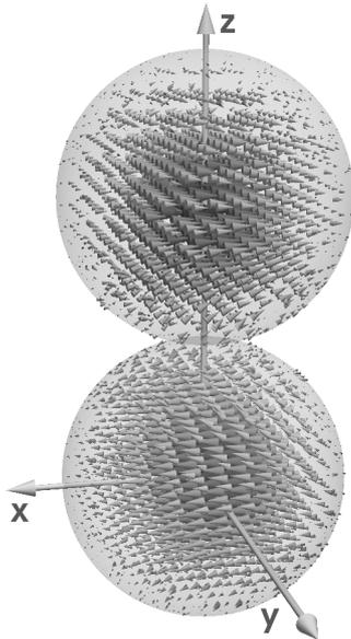
(a) Dipolar mode in a dimer of spheres with radius  $\lambda$  and edge-to-edge distance  $\lambda/200$ .
