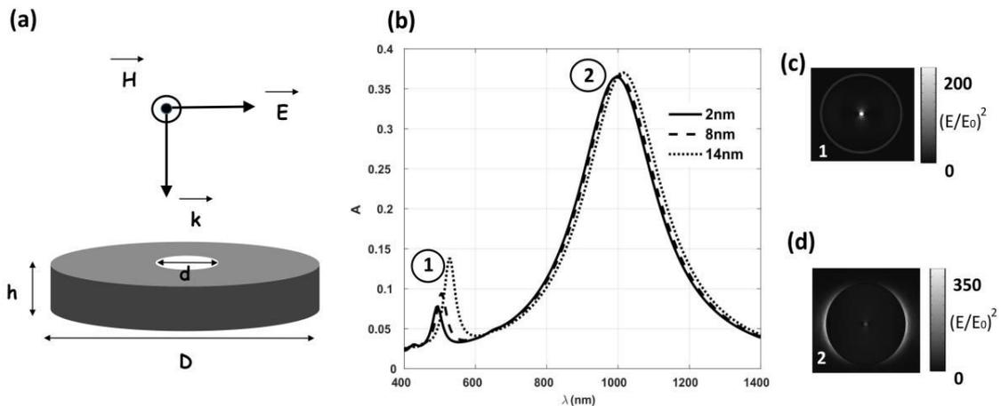
Figure 1: (a) Schematic representation of the 7 nm thickness silver nano-disk of diameter 130 nm with a pore of few nanometer hole at the center. (b) Absorption spectra of a 2,8,14 nm pore diameter. (c) and (d) are respectively the maps of the electric field intensity of resonance (1) and (2) pointed out in (b).
