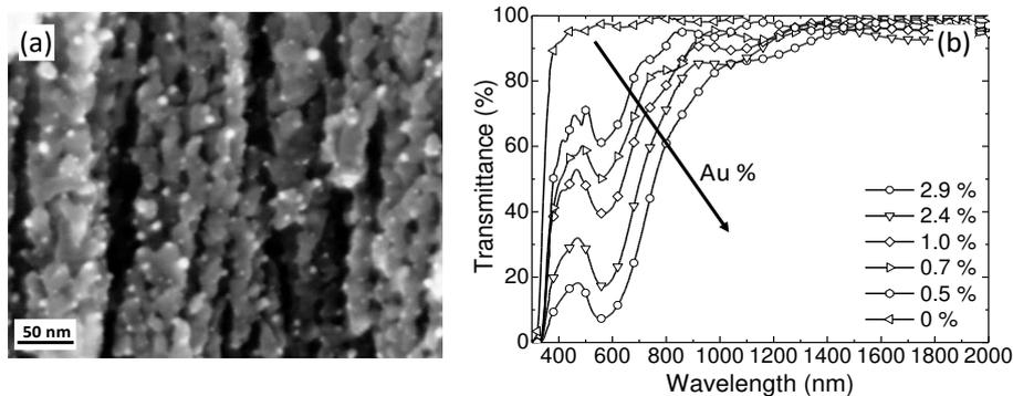
Figure 1: (a) SEM images of Au-TiO<sub>2</sub> integrated structure; (b) Optical transmittance of annealed Au-TiO<sub>2</sub> films with different Au content.
