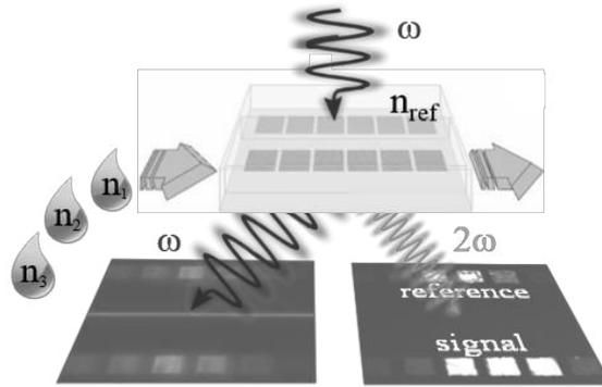
Figure 1: Sketch of the sensing platform. The antenna arrays in the channel are used as sensors, while their reference copy is kept at a constant refractive index  $n_{\text{ref}}$ , under PDMS. The nonlinear emission ( $2\omega$ ) along with the reflectance ( $\omega$ ) from the sensor depends on the refractive index of the flown solutions ( $n_1, n_2, n_3$ ).
