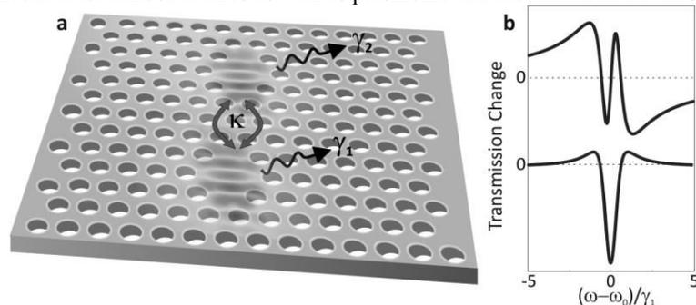
Figure 1. a) Schematics of the photonic molecule under investigation in a photonic crystal slab. The coupling  $\kappa$  was tuned to achieve the closer condition to the exceptional point. b) Transmission spectra in different spots of the photonic molecule near the exceptional point. They exhibit generalized Fano lineshapes.
