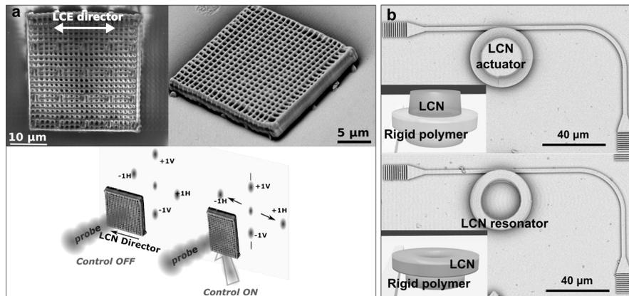
Figure 1: a) Scanning electron microscope (SEM) images of LCN grating beam steerers and light controlled working mechanism. b) On the top, SEM image of the waveguide coupled to Ip-Dip WGM resonator with LCN actuator placed on the top. On the bottom, SEM of the waveguide coupled to LCN ring.
