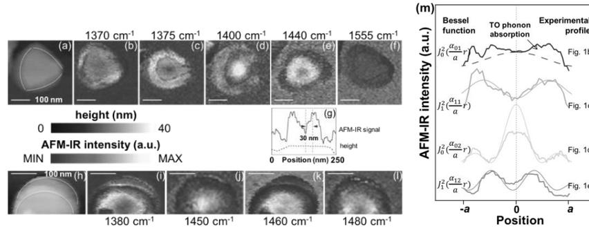
Figure 1: Topography (a and h) and polaritonic standing waves (b-f and i-l) of two samples of hBN with thickness 19 nm and 26 nm, respectively. (g) Amplitude profile of the polariton standing wave of panel (e) showing a lateral resolution of 30 nm. (m) Line profiles of the AFM-IR maps of panels (b-f) and the square of the Bessel functions.
