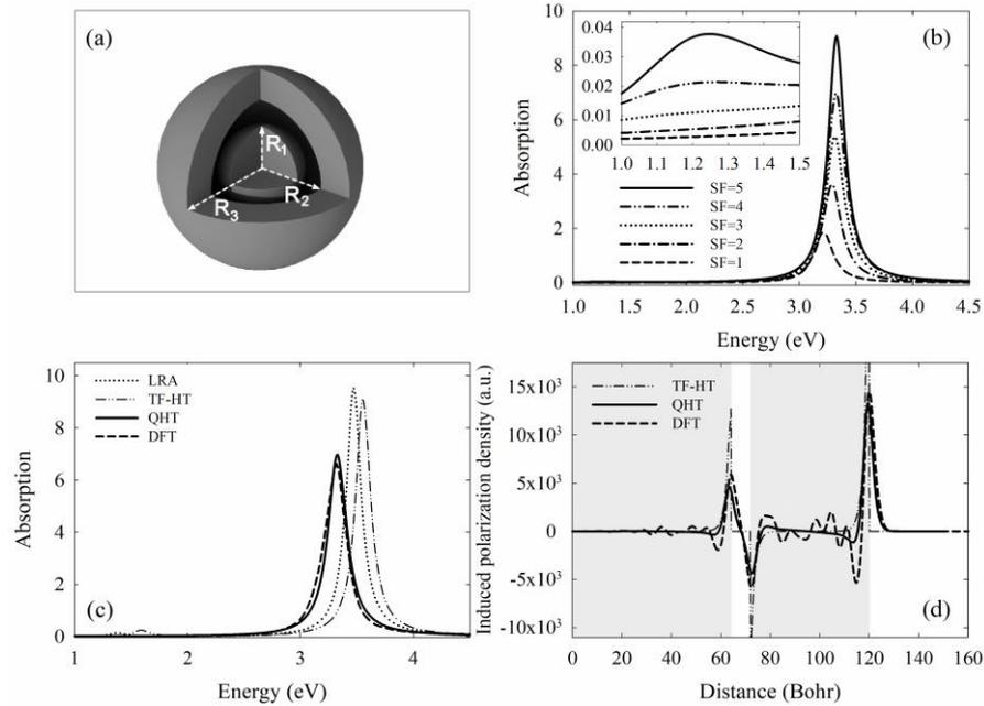
Figure 1: (a) Geometry of the structure (b) absorption spectra calculated using QHT for Na core-shell structures, with the scaling factor ( $SF$ ) taking values from 5 to 1. (c) Absorption spectra and (d) induced polarization density for  $SF=4$  calculated by using different theories.
