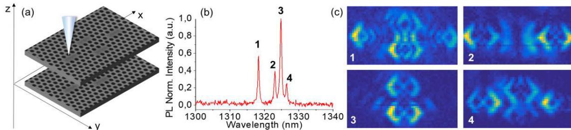
Figure: (a) Sketch of the 4xL3 double membrane structure with near field probe on the left cavity. (b) Experimental near-field photoluminescence (PL) spectrum of a 4xL3 double membrane sample. 1, 2, 3 and 4 indicate the antisymmetric coupled modes of the structure. (c) PL intensity maps acquired at the wavelengths of the 4 modes.
