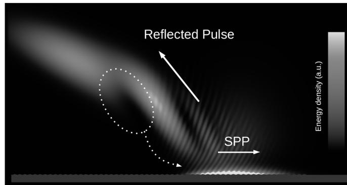
Figure 1: WFR pulse impinging on a grating and generating a SPP. The duration of the latter is proportional to the time in which the resonance condition is satisfied.
