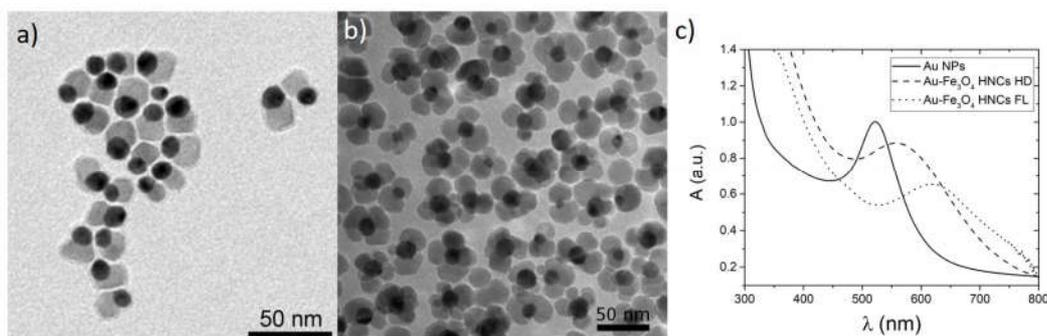
Figure 1: TEM images of Au-Fe<sub>3</sub>O<sub>4</sub> HNCs with a) heterodimer (HD) and b) flower-like (FL); c) UV-VIS spectra of Au-Fe<sub>3</sub>O<sub>4</sub> HNCs with different morphology obtained from iron(III)acetylacetonate.
