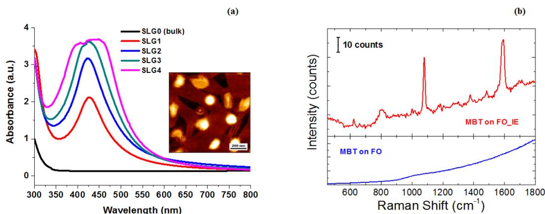
**Fig. 1:** (a) Absorbance spectra of the SLG samples. The inset shows a particular of the SLG4 surface kept by the AFM. The presence of Ag nanoparticles is clearly visible; (b) SERS spectra of the MBT on ion-exchanged (IE) glass fiber optic (FO) tip (red line) compared to the signal acquired by the MBT on the same optic fiber before the ion exchange (blue line).
