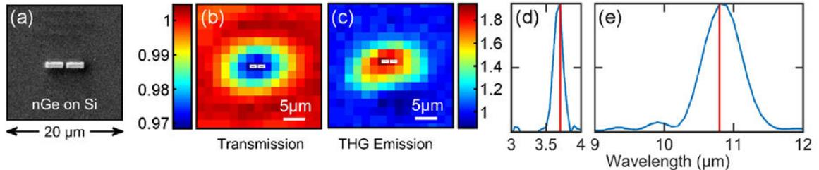
Figure 1: (a) SEM image of a Ge nanoantenna; (b) linear transmission map of a resonant gap antenna illuminated with a central wavelength of 10.8  $\mu\text{m}$ ; (c) THG map normalized to the Si substrate background emission; (d) and (e) normalized THG and excitation intensity spectra, respectively.
