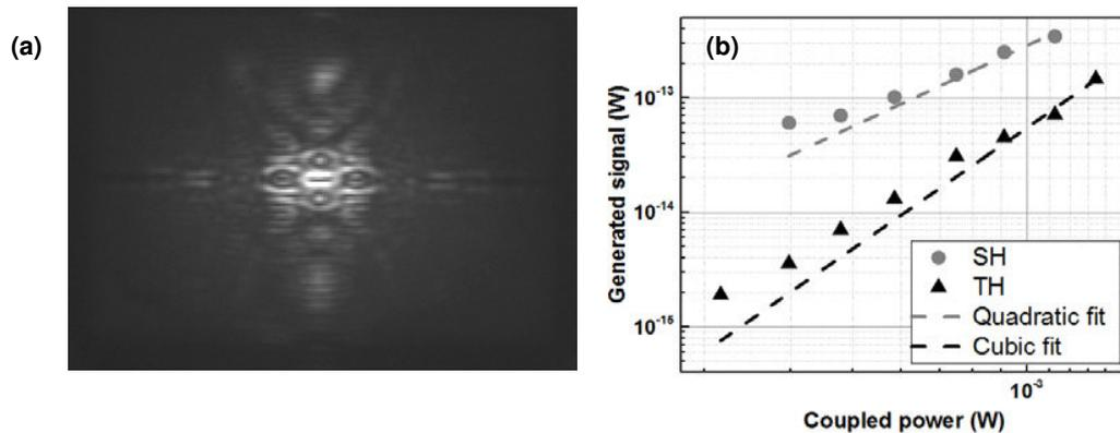
Fig. 1: (a) Image of the generated second harmonic, linear scale. (b) Scaling trends for SH and TH generation.
