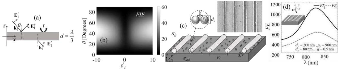
Figure 1: (a) Schematic of longitudinal epsilon near zero film. (b) *FIE* at  $z = (d/2)^-$  as a function of  $\varepsilon'_t$  and incident angle  $\theta$ . (c) The schematic of the proposed “two-scale structure” with rods and plasmonic oligomers. (d) Electric field enhancement for the two-scale structure and linear trimer versus wavelength
