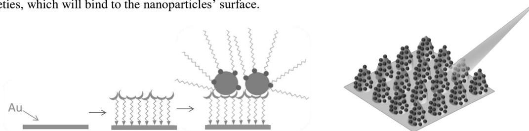
Figure 1: Sketches of the assembly of MNPs on gold nanostructures.
