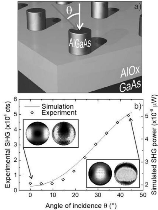
Figure 1: a) Sketch of the fabricated sample of AlGaAs nanodisks on top of a transparent (AIOx) layer. b) Change in the SHG emission with the variation of the incident angle ( $\theta$ , see panel a) of the pump beam, due to a modification of the emission directionality. Inset: theoretical (left) and experimental (right) maps of the back focal plane.
