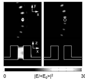
Figure 2. Theoretical analysis of the field distribution within the perforated ring resonator.
