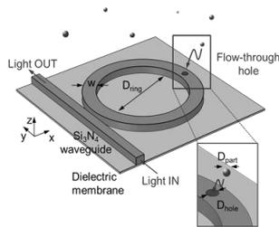
Figure 1. Sketch of the flow-through dielectric ring resonator
