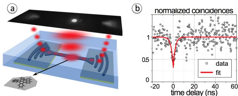
FIG. 1. *Integrated single photon source.* (a) Cartoon of the ridge waveguide and the spin-coated emitters (arrow). On the top, a fluorescence image collected with an EMCCD camera shows signal both at the confocal excitation spot (central) and at the outcouplers. (b) Anti-bunching dip measured at the grating far-field couplers.
