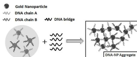
Figure 1: Sketch of the system studied: a solution of gold NPs functionalised with two distinct 12-base DNA chains (A and B) is realised. Then a DNA 24-base 'bridge', complementary to the two sequences, is added to the solution allowing the system to hybridise and to form mesoscopic aggregates.
