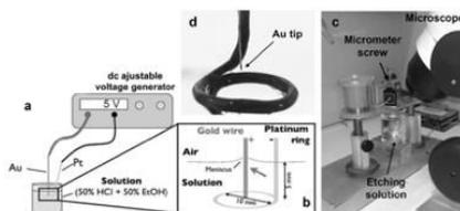
Figure 1: (a) Sketch of the etching experimental setup. The zoomed area (b) shows the details of the tip immersion zone. (c-d) Photograph of the etching setup.
