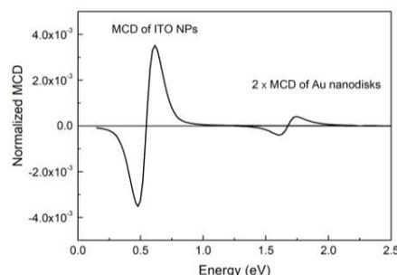
Figure 1: MCD signal of n-ITO NPs compared with that of Au nanodisks.
