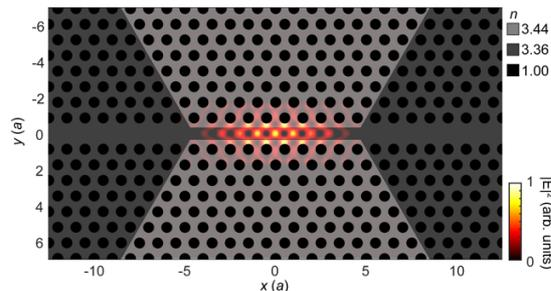
Figure 1: PhC cavity ( $r/a = 0.29$ ) attainable by refractive-index engineering of a GaAsN epilayer (N concentration = 2.2%). The refractive index  $n$  of the untreated (light grey) and hydrogenated (dark grey) material are taken at 1.31  $\mu\text{m}$ . The computed (by FEM calculations) intensity of the electromagnetic field associated with the fundamental cavity mode is superimposed to the structure.
