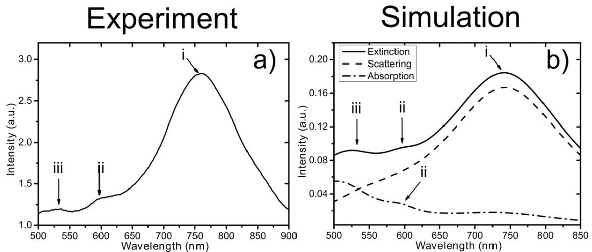
Figure 1. (a) Experimental extinction spectrum of 170nm diameter and 50nm height gold nanocylinder. Illumination is at 50 degree respectively to the normal, (b) corresponding numerical simulation.
