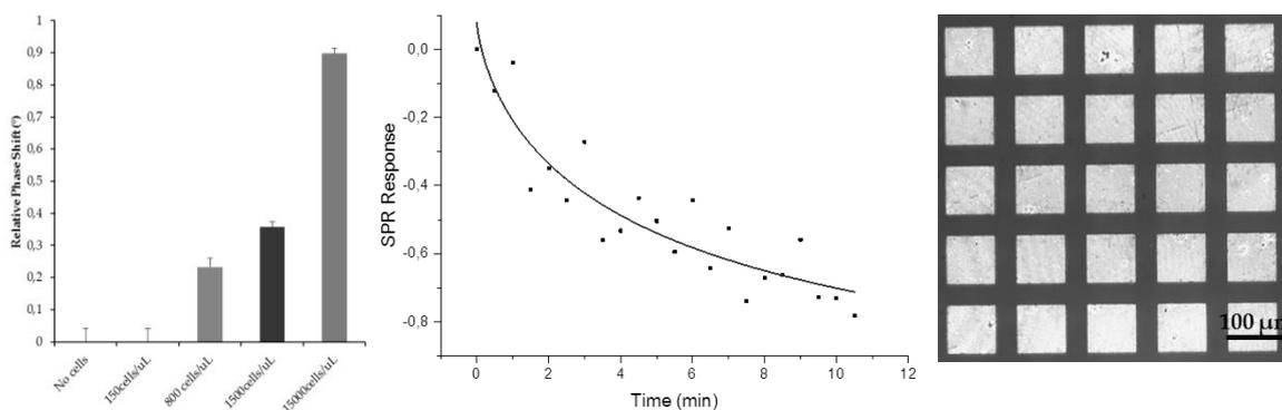
Figure 1. (Left) Calibration between cell number and relative phase shift. (Middle) SPR response decrease upon administration of trypsin to a confluent cell layer. Trypsin has been used as a gold standard for cell detachment from the gold surface. (Right) Optical microscope image of multiplexing of sensing area.
