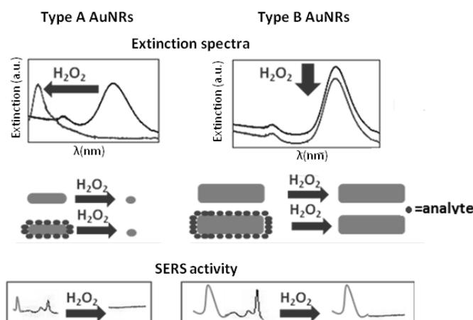
Figure 1. Comparison between the behavior of Type A and Type B AuNRs, before and after the addition of an oxidant: extinction and SERS spectra.
