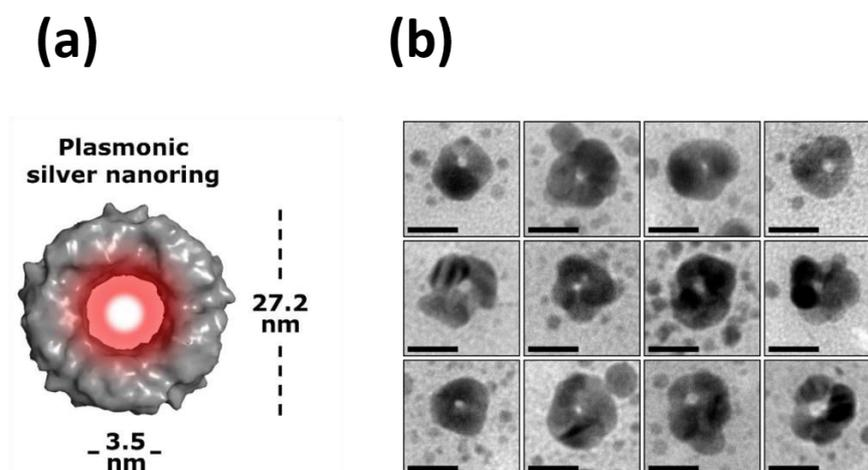
Figure 1: (a) Schematic image of *SmPrxI*-Ag nanoring (b) TEM micrographs at 80 keV of *SmPrxI*-Ag sample after reduction. Mean outer and inner diameters are 27.2 nm and 3.5 nm, respectively. In a number of cases, nanorings are found decorated with small particles. Scale bars= 10 nm.
