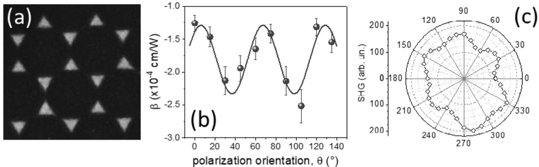
Figure 1: (a) SEM image of a nanoprism array. (b) Nonlinear absorption coefficient ( $\beta$ ) as a function of the linear polarization orientation. (c) Polar plot of the polarization-dependent SHG signal.
