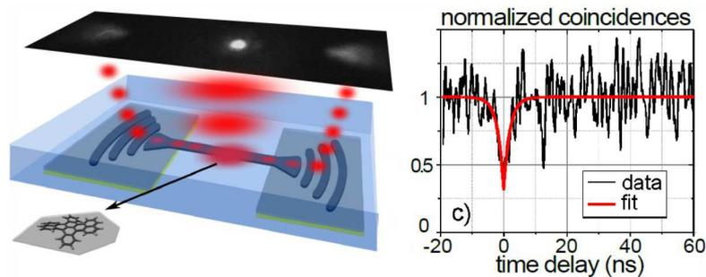
Figure 1: Cartoon and fluorescence image collected with an EMCCD camera showing signal from both the confocal excitation spot and the outcouplers; antibunching dip measured in correspondence of all output ports reveals single-photon nature of the signal.
