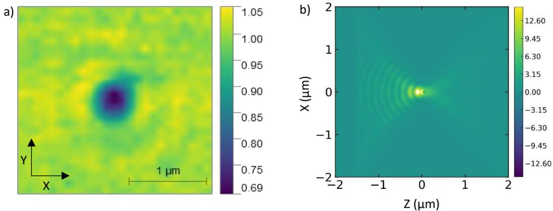
Figure 1: a) Raw iSCAT image of a 60 nm GNP immobilized on functionalized glass. Colour scale represents iSCAT contrast. b) Simulation of distribution of  $|E|^2$  electric field injected at  $Z = -1.5 \mu\text{m}$  and focused on GNP.
