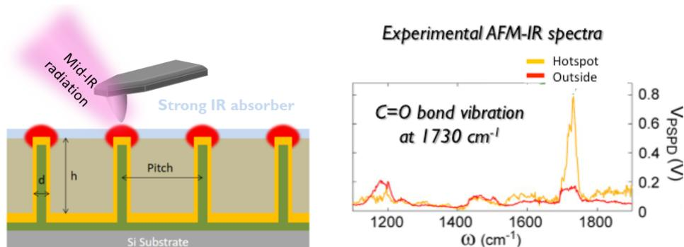
Figure 1: Left: scheme of the experimental setup for detection of the local photothermal expansion (Ansys NanoIR2 with MIRcat Quantum Cascade Laser). Right: AFM-IR spectra demonstrating the vibrational absorption enhancement for the C=O bond of PMMA resonant with the antennas.
