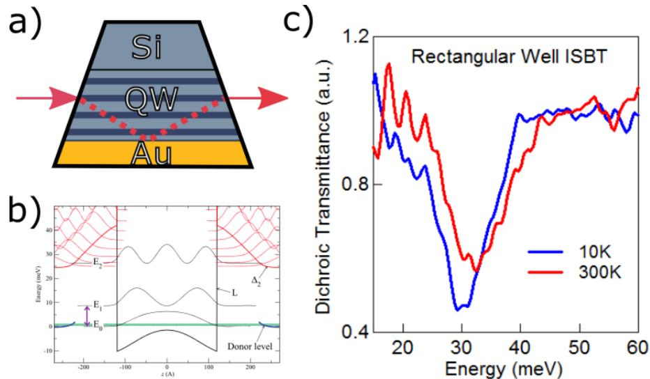
Figure 1: a) Schematic representation of the single-plasmon waveguide geometry used for measurements. Red arrows represent light coming in and out of the sample. b) Square modulus of the wavefunctions and energy levels of a rectangular quantum well. c) ISBT in a rectangular QW measured by Fourier-Transform IR spectroscopy
