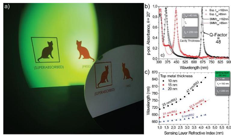
Figure 1: (a) Colour change of the p-polarized image of a cat in a box that turns black on the screen due to the superabsorption of its original red colour, in contrast to the non-polarized one that remains black. (b) MIM based superabsorber and (c) refractive index sensor.
