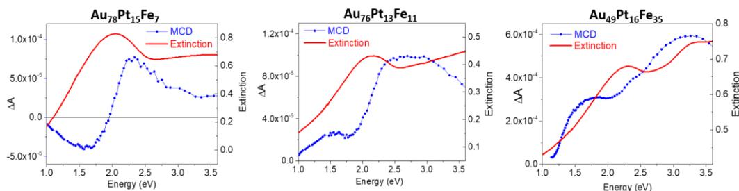
Fig. 1 : MCD spectra (blue) at 1.4 Tesla, and extinction spectra (red) of three AuFePt nanoalloys with different composition, dispersed in a polymer film.
