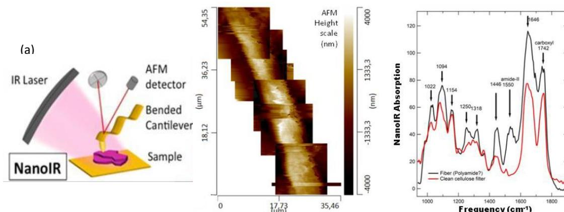
Figure 1: (a) Sketch of the AFM-IR instrument. (b) AFM image in contact-mode of a micro-fiber found on a cellulose filter through which seawater was passed. (c) NanoIR absorbance of the micro-fiber (black line) compared to the absorbance of the clean cellulose filter surface (red line).
