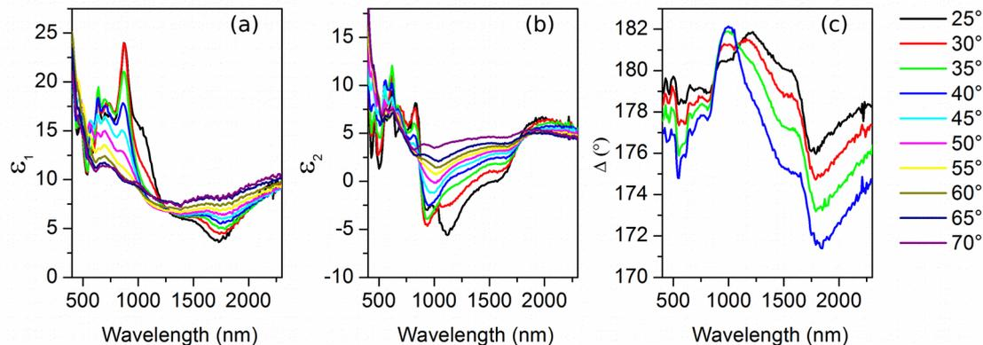
Figure 1: (a)  $\epsilon_1$ - and (b)  $\epsilon_2$ - pseudo-functions and (c)  $\Delta$  measured for a Golden Angle Vogel spiral distribution of gold capped Silicon cylinders.
