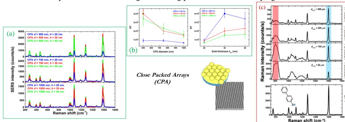
Figure 1: (a) BPT SERS spectra of hexagonally CPA structure with nanospheres diameters,  $d = 500, 750, 1000$  nm and gold film thickness,  $t_{Au} = 20, 30, 40$  nm. (b) EF as function of the CPA diameter and gold thickness, respectively. (c) Raman spectrum from 100 mM BPT solution through different optical fibers and Raman spectrum from the BPT solution with the Raman microscope without the fibers.
