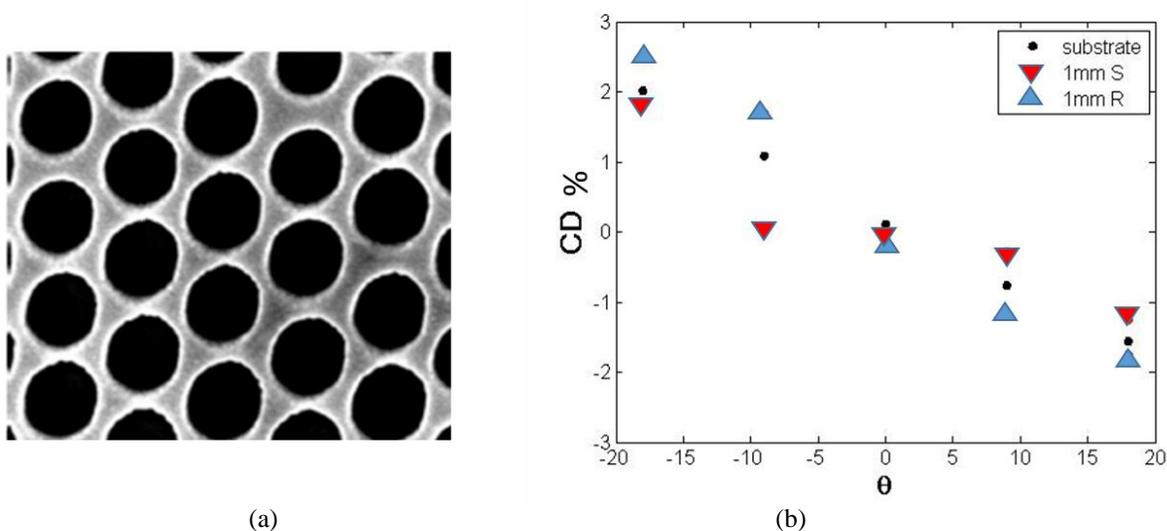
Figure 1: (a) SEM image of the realized sample. (b) circular dichroism as a function of incidence angle of the bare substrate (black circles), right-handed molecules on the substrate (blue triangles), left-handed molecules on the substrate (red reversed triangles).
