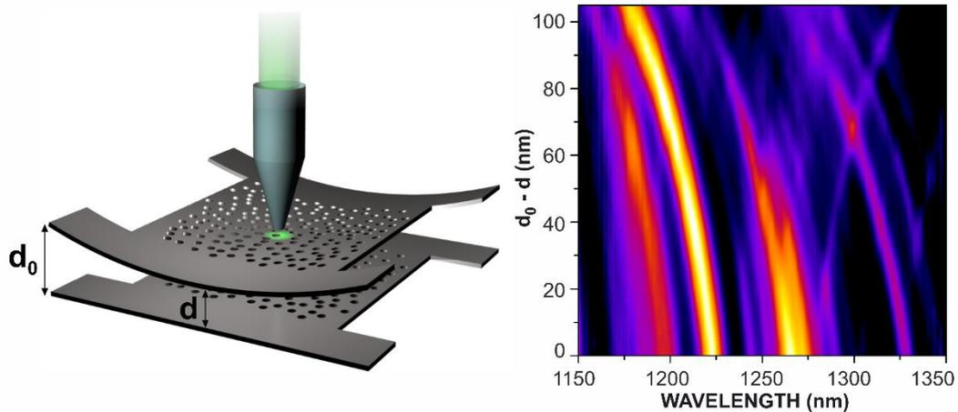
Figure 1: Sketch of the double membrane tip compression, where we exaggerated the bending for sake of illustration. Typical spectra (with many modes), reported in a color map, at different double membrane compression. Note the dominance of asymmetric modes, but also the presence of one symmetric mode on the long-wavelength side.
