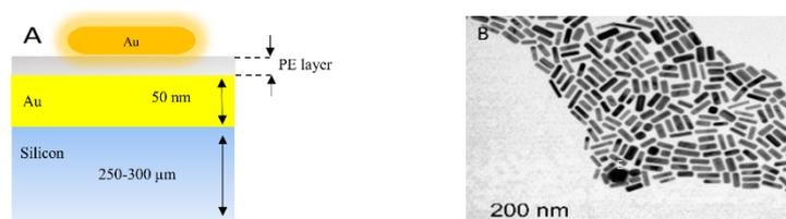
Figure 1: Au nanorods over a Au film (A). TEM images of GNRs as fabricated (B).
