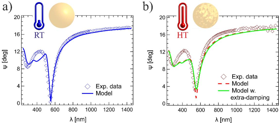
Figure 1: Experimental ellipsometric spectra (markers) and calculated curves (lines) at a) room temperature (RT) and b) high temperature (HT). Agreement at HT is improved by considering an extra-damping contribution in the model (green curve).
