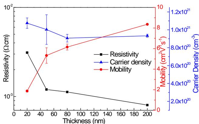
Fig. 1: Carrier density, mobility and resistivity of PLD Ta:TiO<sub>2</sub> films as a function of film thickness (5% at. Ta content, 1 Pa O<sub>2</sub> deposition pressure).
