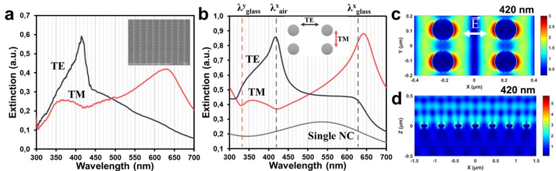
Figure 1: Experimental (a) and simulated (b) extinction spectra of the Al nanoparticles array (lattice 420x216 nm) for two orthogonal polarizations. Calculated extinction spectrum of the single Al nanocylinder on glass ( $d=150$  nm,  $h=50$  nm) (b). Electric field maps for the polarization along the X axis at the resonance wavelength (420 nm) in XY (c) and XZ (d) cuts.
