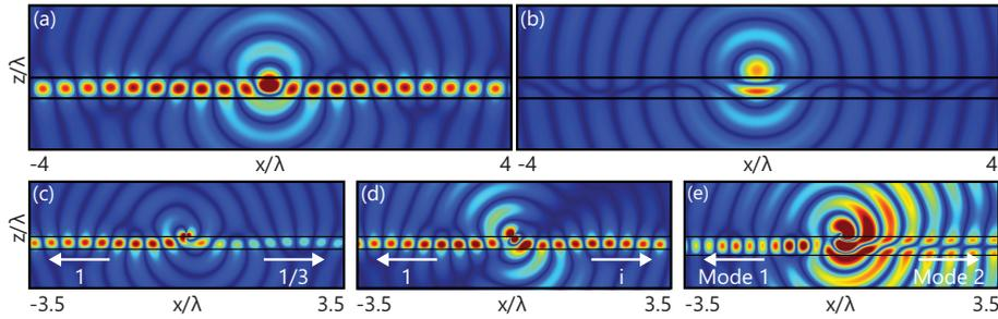
Figure 1: Magnetic field of a coupling (a) and noncoupling (b) Janus dipole placed near a single mode waveguide. In (c), (d) and (e), a multimode waveguide is excited in opposite directions with three different dipolar sources, which (c) couple to the same mode with different amplitudes, (d) couple to the same mode with opposite phases and (e) couple to two different modes.
