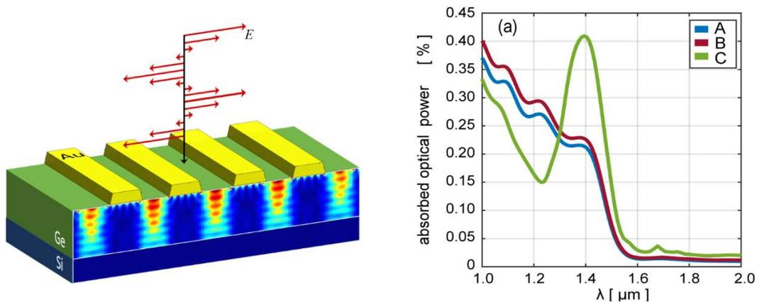
Figure 1: Left: Cartoon of a metallic grating. Au and Ge layers are depicted in yellow and green, respectively. Normal illumination and an electric field polarization orthogonal to the metal grating elements are taken into account. The color map reports the simulated absorption. Right: The simulated absorption spectra vs.  $\lambda$  of the resonant (C) and not resonant (A and B) MSM photodetectors.
