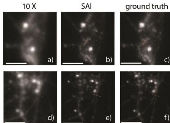
Figure 1 a-d: Images obtained of a cortical neuron taken with a low numerical aperture objective (NA=0.25). b-e: Super resolution images obtained with the same objective (NA=0.25) and Scattering Assisted Imaging deconvolution. c-f: Ground truth obtained with a high resolution objective (NA=0.75).
