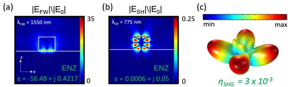
Figure 1: Electric field enhancement at the Fundamental Wavelength (FW) [(a)] and Second Harmonic (SH) [(b)] in the case of nanocylinder with radius  $r$  and height  $h$  placed over the ENZ. The permittivity of the ENZ substrate is also indicated. (c) The SH Far Field.
