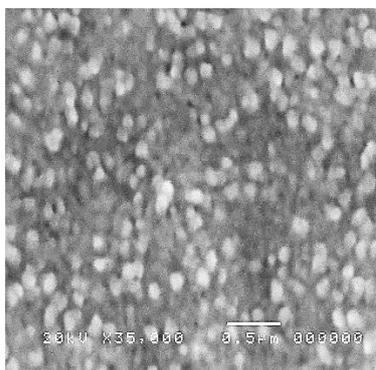
Figure 1: Dewetting of an Ag layer @60 nm deposited on a silicon wafer after oxidation, induced by 2:30 minutes of plasma treatment. The bar scale corresponds to 0.5  $\mu\text{m}$ .
