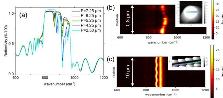
Figure 1: (a) Far field reflectivity spectra of SiC pillar arrays with different array pitches  $P$ . Near-field signal on a line along the top of a pillar (b) and along the SiC surface between pillars (c), showing frequency modulations that are otherwise obscured by far-field averaging.
