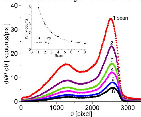
Figure 1: Fluorescence angular spectra acquired after successive scans. (in the inset: the integrated fluorescence signals over the scans).
