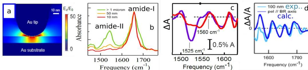
Figure 1: (a) Simulation of field enhancement in the 10-nm wide plasmonic nanogap. (b) AFM-IR absorption spectra of BR. (c) Difference AFM-IR  $\Delta A$  under visible light stimuli on a 1 micron thick film (purple) and on the 10-nm thick membrane stack in the nanogap (red). (d)  $\Delta A/A$  comparison with theory.
