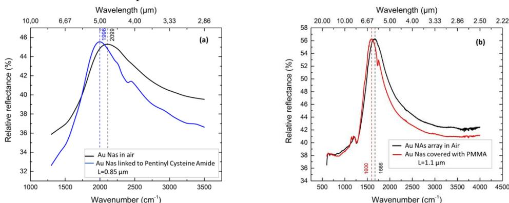
Figure 1: Reflectance curve of NAs array (black) in air versus reflectance curve (blue) of NAs array linked to Pentynyl Cystein Amide (a) and reflectance curve (blue) of NAs array covered with a 50 nm PMMA layer (b).
