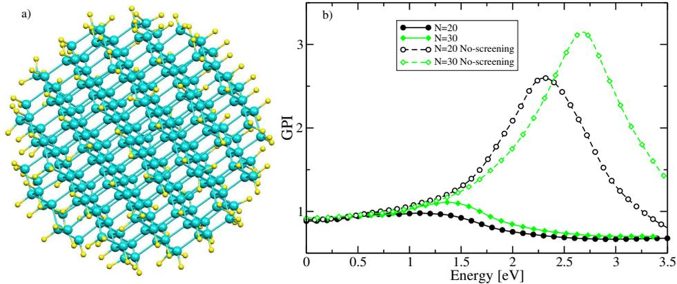
Figure 1: a) Atomic structure of one of the considered silicon NC. The surface atoms have been passivated with hydrogen atoms. b) GPI for a NC with different number ( $N$ ) of excess electrons: the GPI increases (and blue-shifts) with  $N$  and it is much larger (and blue-shifts) when the interaction with the valence electron is switched off (no screening).
