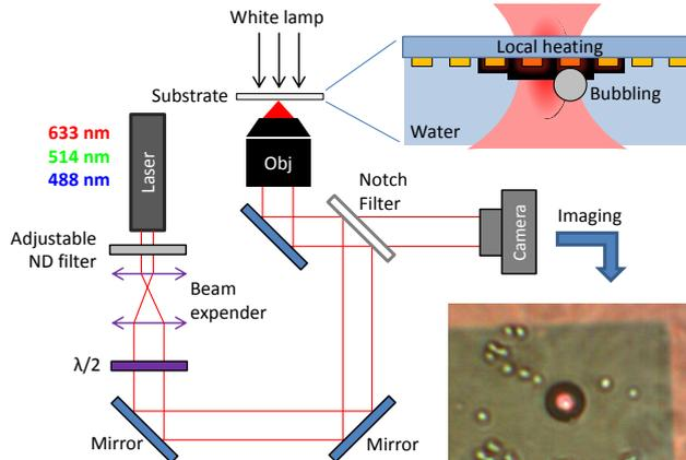
Figure 1: Experimental setup used to excite plasmons and visualise induced bubbling.
