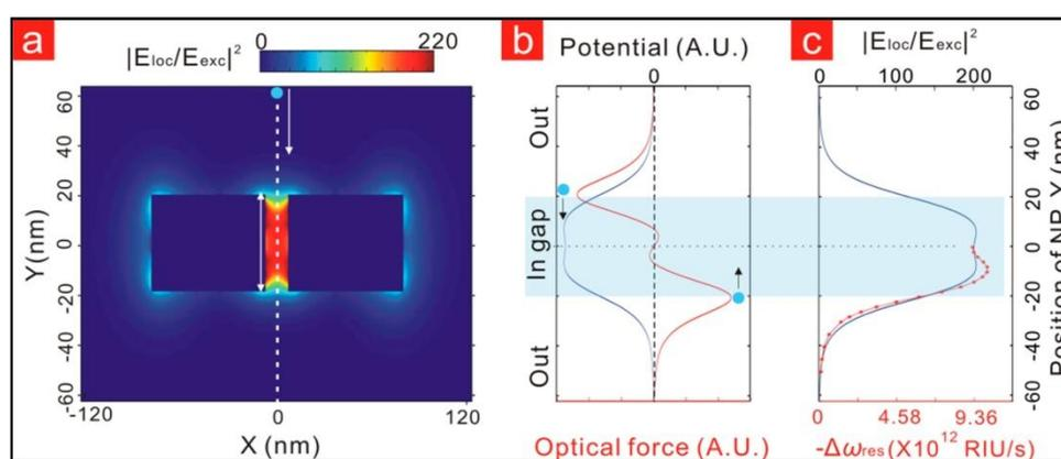
Figure 1: (a) Local field intensity plasmonic dimer nanocavity. (b) Optical force and trapping potential of the nanocavity. (c) Relationship between trapping-induced resonance frequency shift (red) and associated potential energy (blue) of the nanocavity upon trapping of small nanoparticle [3].
