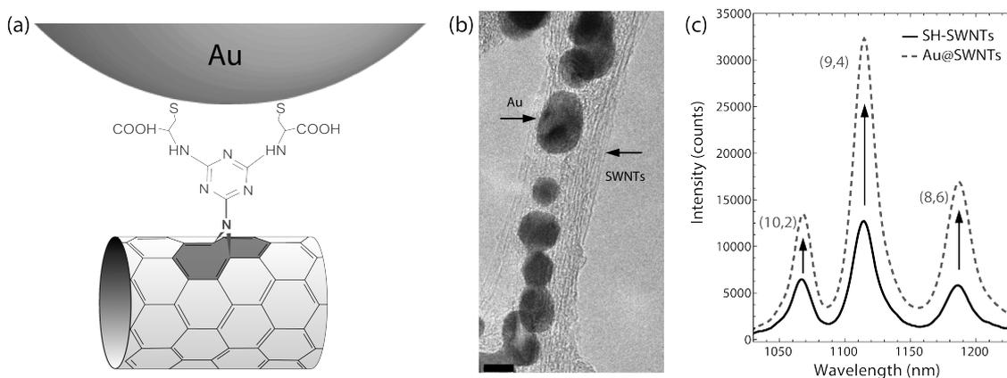
Figure 1: (a) Molecular sketch of AuNPs covalently anchored to thiol-functionalized SWNTs. (b) TEM micrograph of Au@SWNTs hybrids. Scale bar, 5 nm. A few-SWNTs bundle can be observed as well as AuNPs assembled along the tubes. (c) Enhancement of the luminescence emission of SWNTs after covalent attachment of AuNPs onto their surface: Comparison of the emission of the Au@SWNT hybrids (dotted curve) with the one of SH-SWNT (black curve). Picture adapted from [2].
