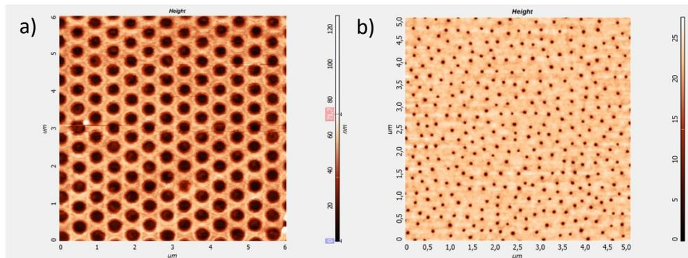
Figure 1: AFM topography of long-range (a) and short-range (b) ordered NH.
