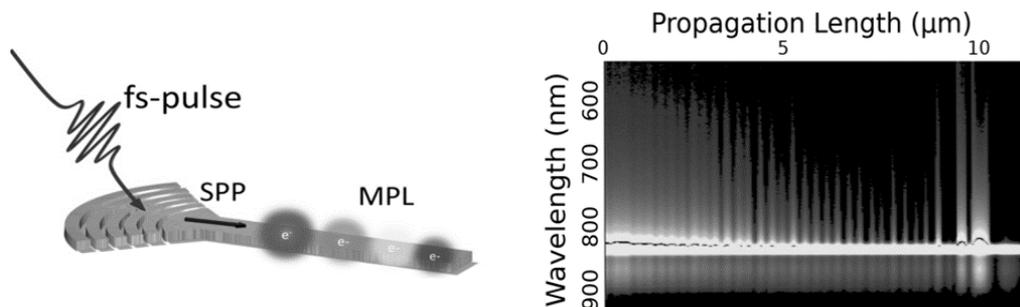
Figure 1 (left): Plasmonic waveguide with grating coupler showing SPP propagation and hot-electrons relaxing emitting MPPL. Figure 2 (right) : Hyperspectral near-field measurement showing the spectral variation of MPPL along the propagation of SPP
