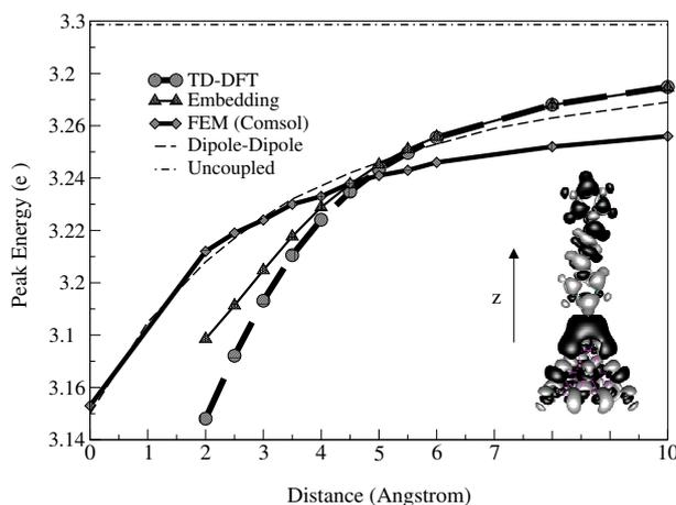
Figure 1: Bonding mode energy vs metal-molecule distance for the four applied methods. Inset: transition density at the bonding mode resonance for  $d = 2 \text{ \AA}$ .
