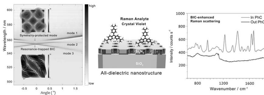
Figure 1: The dispersion diagram of the metasurface (left) reveals the existence of normal-incidence BICs, used to amplify the local optical field in proximity to the surface (center) for Raman scattering enhancement (right).
