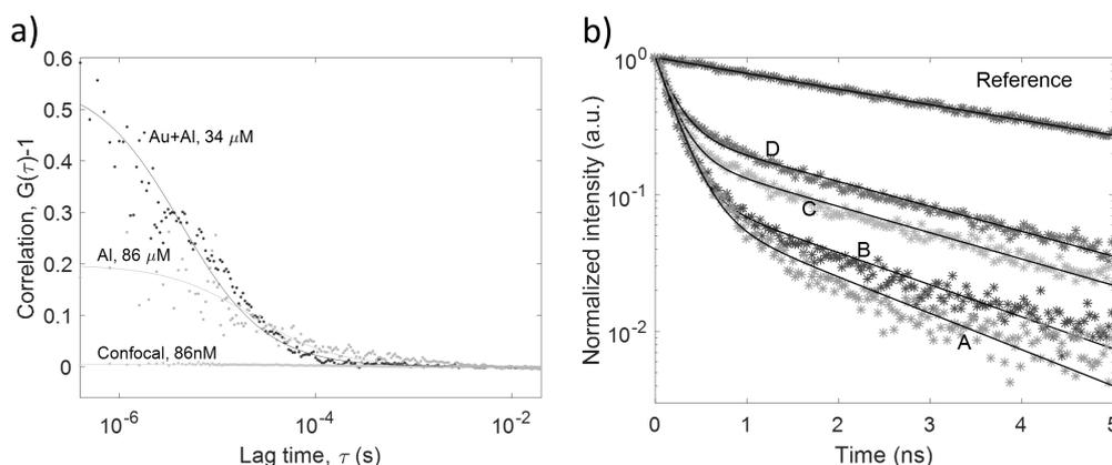
Figure 1: a) FCS measurements using ZMWs. b) Lifetime measurements using PNs.
