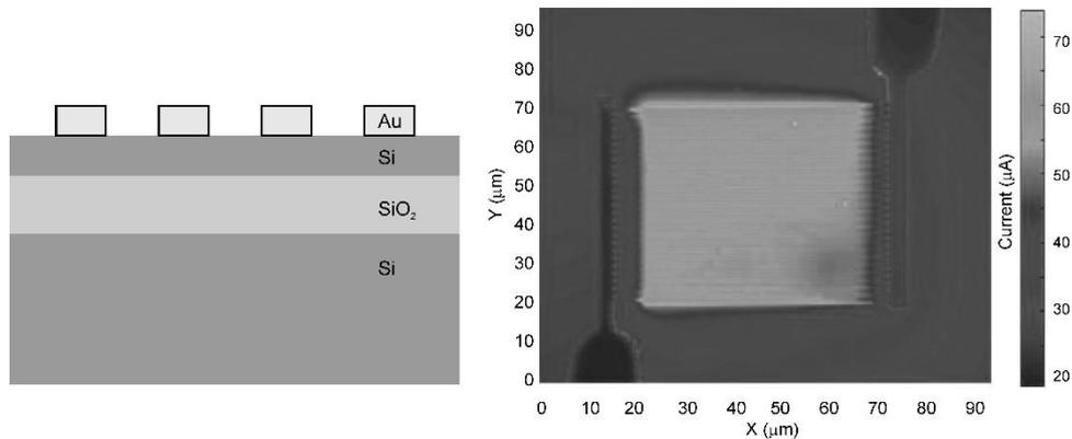
Figure 1: Sketch of the investigated device (left) and preliminary photocurrent mapping at 790 nm wavelength with 3 mW power and 0.5 V bias (right).
