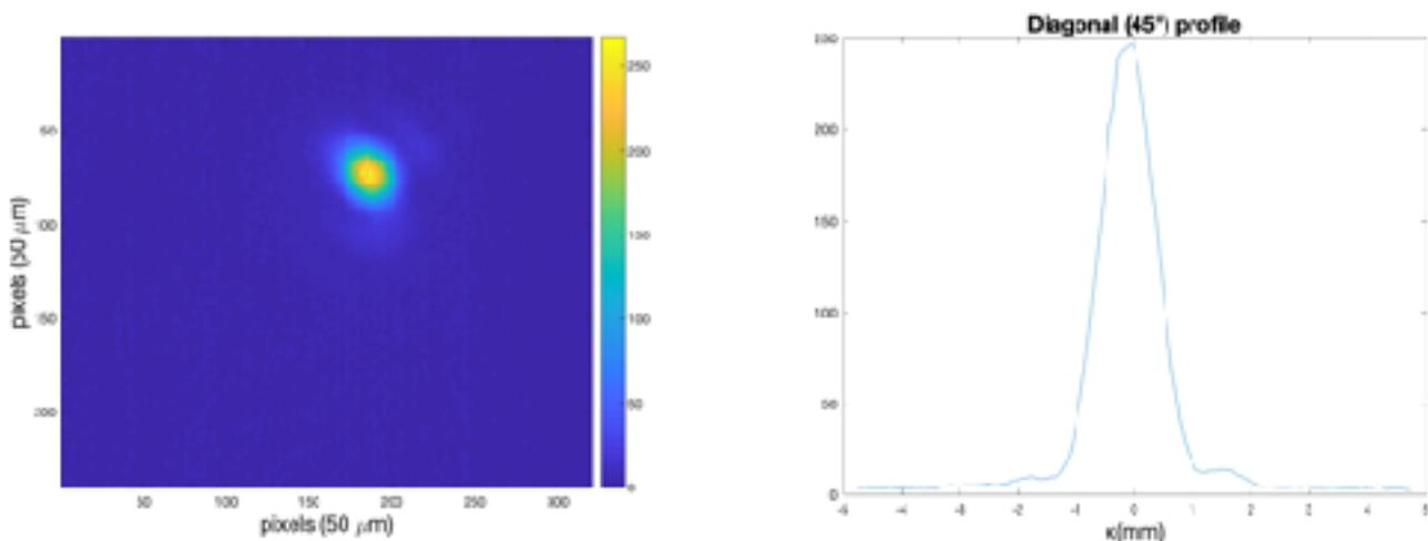
**Fig. 1** On the left: focal spot on a terahertz camera of the beam reflected by a skin simulant sample. On the right: the plot shows a line profile along the diagonal (45°) direction. Intensity in ADC counts.
