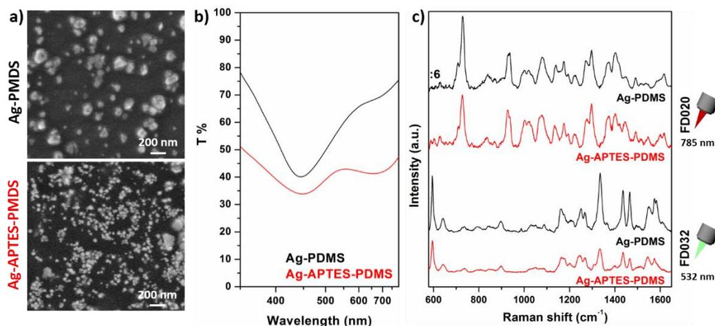
Figure 1: a) FESEM images, b) UV-Vis-NIR transmission spectra and c) SERS spectra of NIR and green cyanines dyes (FD020 and FD032, FLUODY S.r.l.) ( $10^{-5}$  M, resonantly excited at 532 and 785 nm, respectively) obtained from the best performing Ag-PDMS substrates (40 °C, 24 h in 100 mM AgNO<sub>3</sub>).
