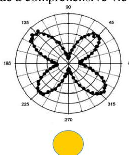
Figure 1 : Polar plot of the Second Harmonic Scattering intensity polarized perpendicularly to the plane of scattering recorded for an aqueous suspension of dispersed 150 nm gold nanospheres.
