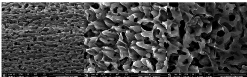
Figure 1: SEM micrographs of the porous aluminum material. Different areas of the same sample.
