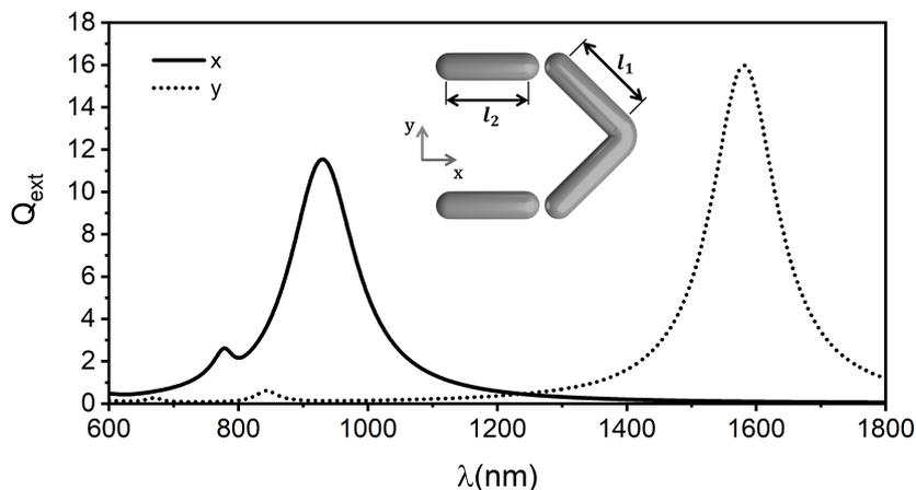
Figure 1: Scattering spectrum of the plasmonic nanostructure: straight and dot lines represent the linear extinction efficiencies of the coupled antenna, calculated using FEM method, when illuminated with light polarization parallel (x-axis) and orthogonal (y-axis), respectively, to the nanorods. Inset: doubly-resonant gold nanostructure designed for efficient DFG.
