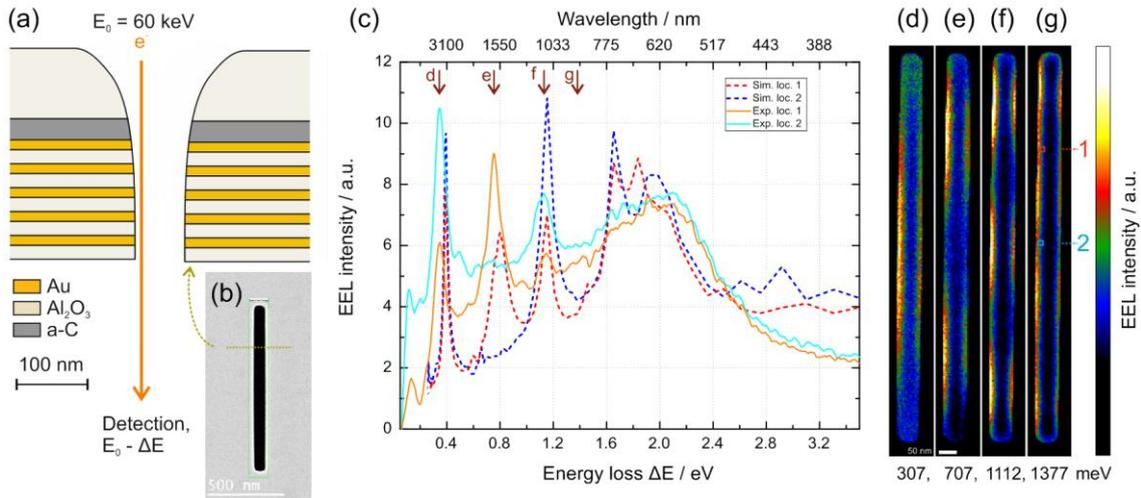
Figure 1: HMM slot resonator, length 1  $\mu\text{m}$ . a) Cross-section schematic of the measurement. b) High-angle annular dark field STEM image of the slot. c) Simulated and experimental EELS spectra at two positions marked in g) with resonant peaks marked and the zero-loss peak subtracted. d-g) Experimental EELS intensity maps of the same slot at the marked energy losses.
