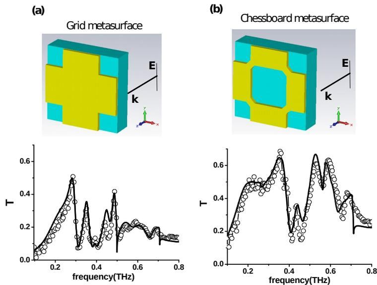
Figure 1: geometrical sketch of the unit cell and transmission properties of a GR (a) and a CB (b) metasurface. Open circles describe the experimental results whereas black continuous lines represent full wave electromagnetic simulations.
