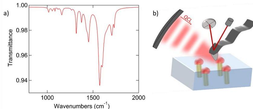
Figure 1: a) Transmittance of 2.2 $\mu\text{m}$ -thick evaporated CaF<sub>2</sub> film measured by Fourier Transform InfraRed spectroscopy in the fingerprint region. b) Pictorial sketch of the nanoIR setup used for the measurements.
