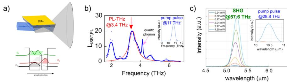
**Figure 1:** a) Sketch of the 70° surface plasmon waveguide configuration used for both the PL experiment performed on n-doped ACQWs and the SHG experiment on p-doped ACQWs. A PL spectrum and a SHG spectrum are also reported in panel (b) and (c), with the FEL pump pulse and the OPA pump pulse as insets, respectively.
