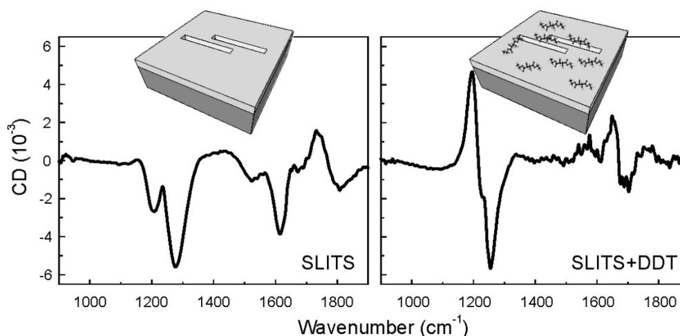
Figure 1: Representative CD spectra from clean slits (left) and slits covered with DDT (right).
