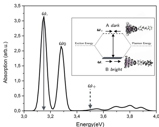
Figure 1: TD-DFT absorption spectrum of the whole system for the metal-molecule distance of 2 Å. In the inset, a pictorial scheme of the coupling between a plasmon and an exciton. All the calculations have been performed with TURBOMOLE code [2].
