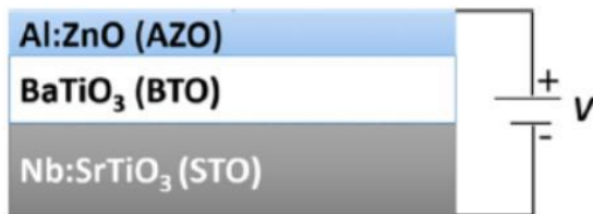
Figure 1: Proposed MOS capacitor architecture for gating of the AZO film.
